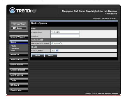
The Web Configuration contains the settings that are required for the camera in the left menu bar, including Smart Wizard, Basic, Network, Video/Audio, Event Server, Motion detect, Event Config, Tools, SD Card, and Information.
